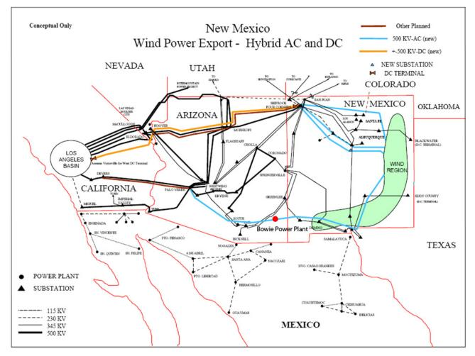
SWAT's original conceptual map to export New Mexico wind-generated electricity. The southernmost 500-kV line that SWAT proposed passed through the SouthWestern Power Group's permitted Bowie power plant, prompting SWPG to propose SunZia to serve both the plant and SWAT's purpose.
