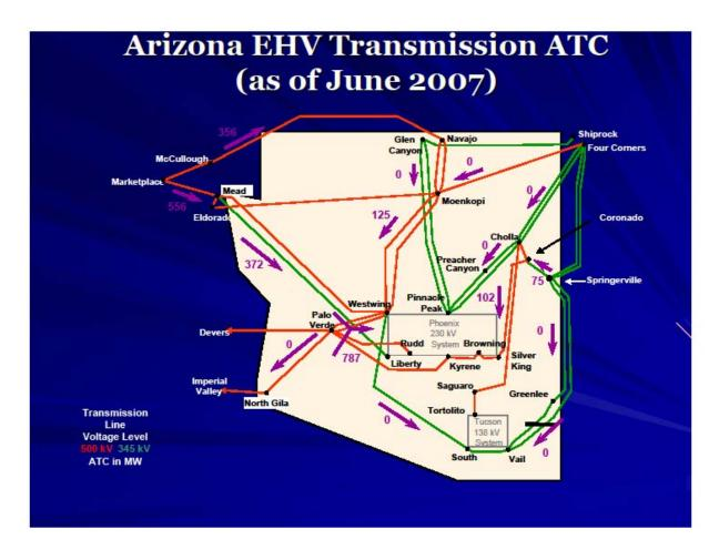
Group of transmission capacity means that TEP would at times have to limit the power it uses from its own Springerville generating stations.
